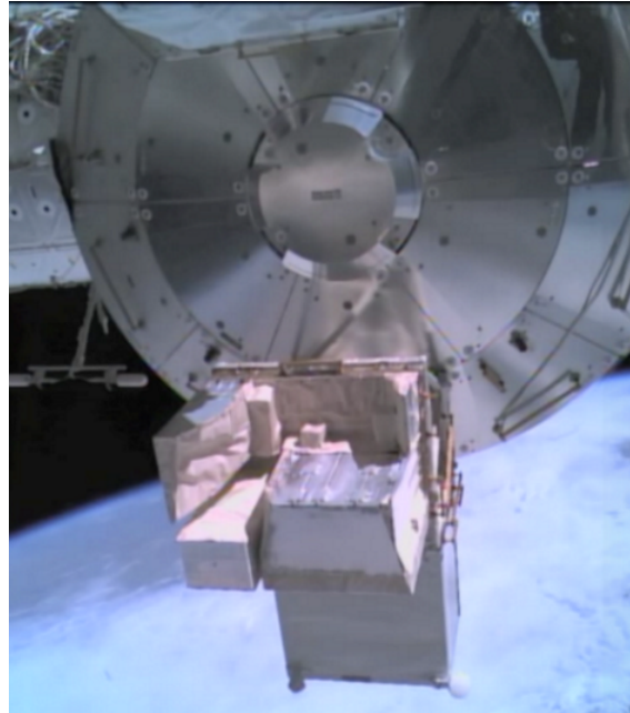
Figure 1: Figure 1: ACES installed at the external payload facility of the Columbus module and pointing towards the Earth (Credits: @ESA-NASA).
