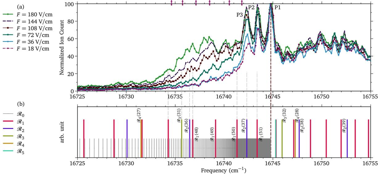
Figure 1: (a) Normalized  $\text{Rb}_2^+$  ion count as a function of the second photon frequency for several electrical fields ( $F=180, 144, 108, 72, 36,$  and  $18 \text{ V/cm}$ ). (b) Rydberg states associated with the vibrational levels of  $^{85}\text{Rb}_2^+, X^2\Sigma_g^+, v^+ = 0, 1, 2, \dots$  labeled as  $\mathcal{R}_0, \mathcal{R}_1, \mathcal{R}_2 \dots$ , respectively.
